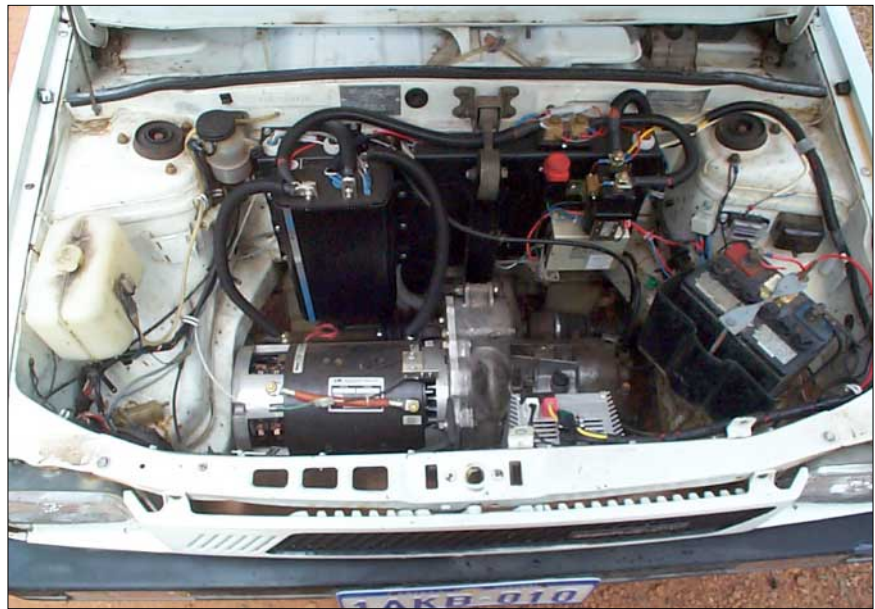
Inside the engine bay. Note how small the electric motor is compared to a petrol engine.
