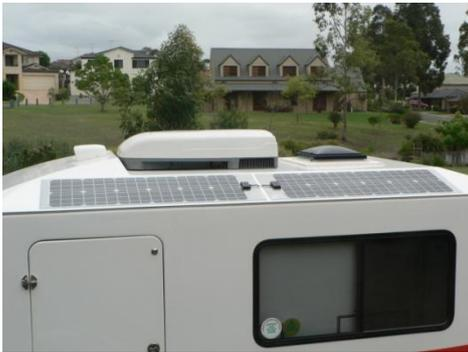
In addition to the Karavan's own Ranox powered by the tug and providing up to 25 amps if necessary, there are four 50 watt panels on the Karavan roof in a series-parallel arrangement feeding a GSL MPPT 30-2 solar regulator..
