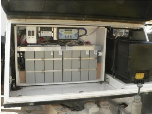
The picture to the left shows the battery box (cover removed), the new 360 Ah lithium batteries and above them their BMS and the GSL's remote display. The regulator itself can be seen to the top right of the battery box. Its LOAD socket, referred to elsewhere, is hidden from view.
