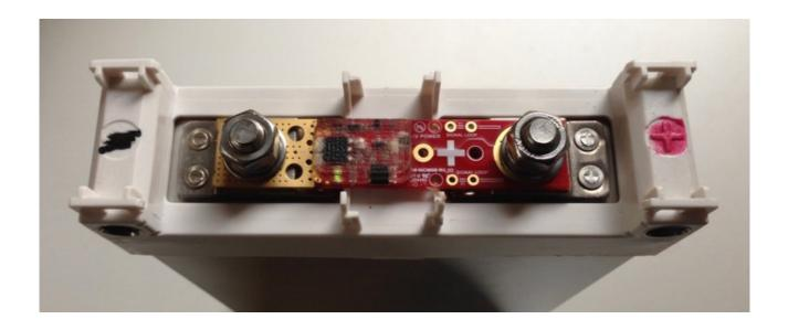
EV power CBM cell balancing/monitoring modules combine simplicity and reliability to maintain Lithium NCM (Nickel Cobalt Manganese) cell balance and protection.
