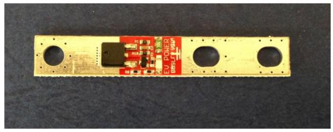
NOTE: The module can be easily cut to fit 20Ah cells by using metal cutting shears.
