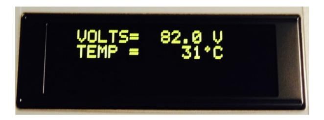
Press the button on the Configurator and the display will show Stack 1 voltages, up to 12 cells, and temperature as below. Scroll through up to 4 stacks this way. The cells are in groups of three with labels A,B,C, D.
